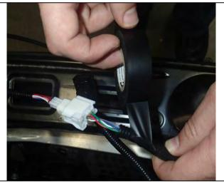
13. Apply electrical tape to insulate exposed areas of loom and hold convoluted tube as shown.
