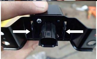
2. Separate OEM steel bracket from back of camera by removing two Philips head screws and depressing shroud clips.
