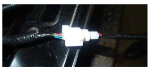
14. Plug the supplied camera loom into the connector (now part of vehicle loom) and route down under the grill so it can be plugged into the camera.
