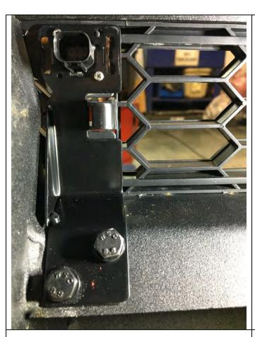
6. Using supplied hardware, attach bracket and camera to bar.
